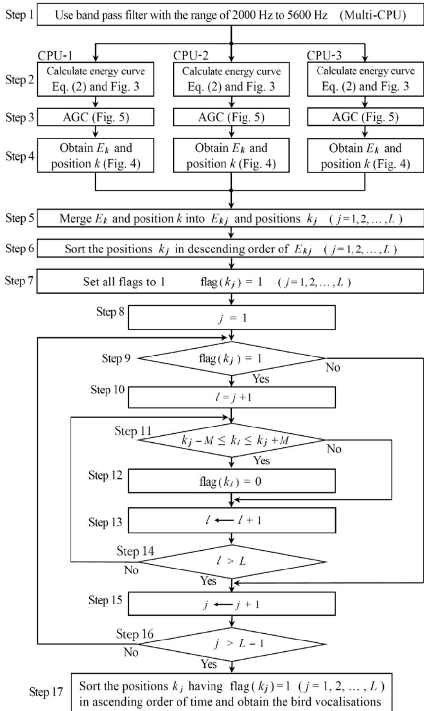
Fig. 6 Flowchart for segmentation
