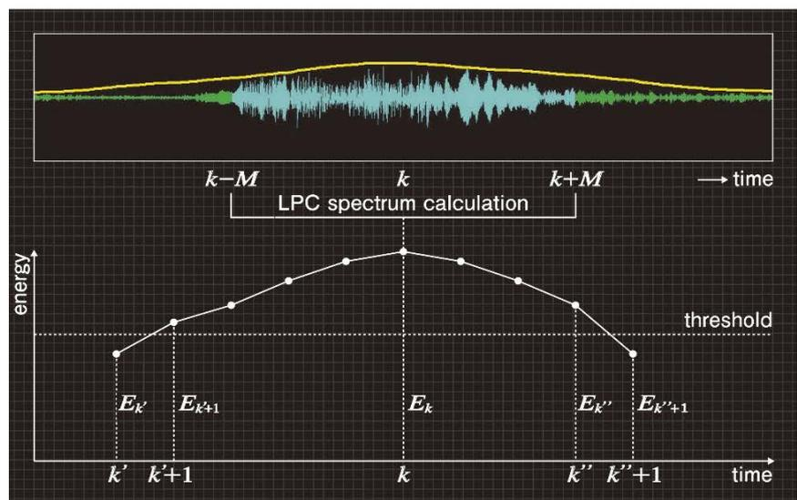
Fig. 4 Comparison of energy curve with threshold
