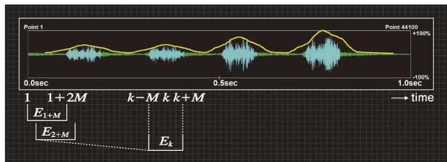
Fig. 3 Calculation of energy curve
