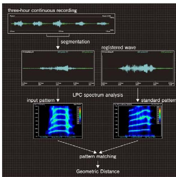
Fig. 2 Processing procedure in recognition system
