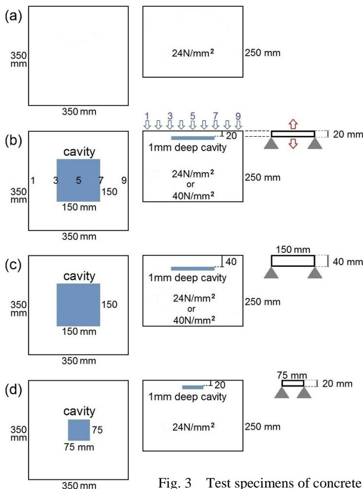
Fig. 3 Test specimens of concrete
